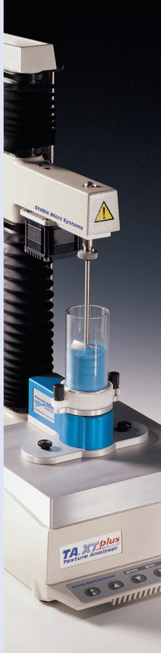
Fig 2: Cohesion Test for Non Bio Washing Powder
