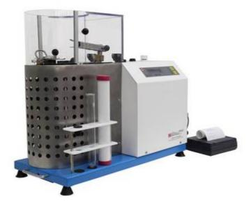
The instrument is microprocessor controlled and includes a shaking mechanism associated to temperature regulated water bath. The water bath needs no external cooling water as the water level is kept constant by a built-in water tank.
